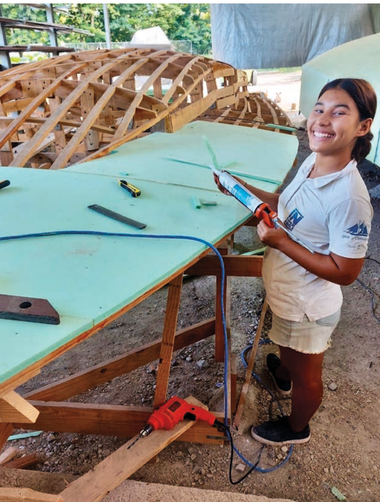
Above, Alice Bianchetti, Pui and Raoul’s 15-year-old daughter, smiles while working on the deck. Opposite page: To save money and control quality, Jordan and Raoul opted to build the hull and deck molds over wood frames.
